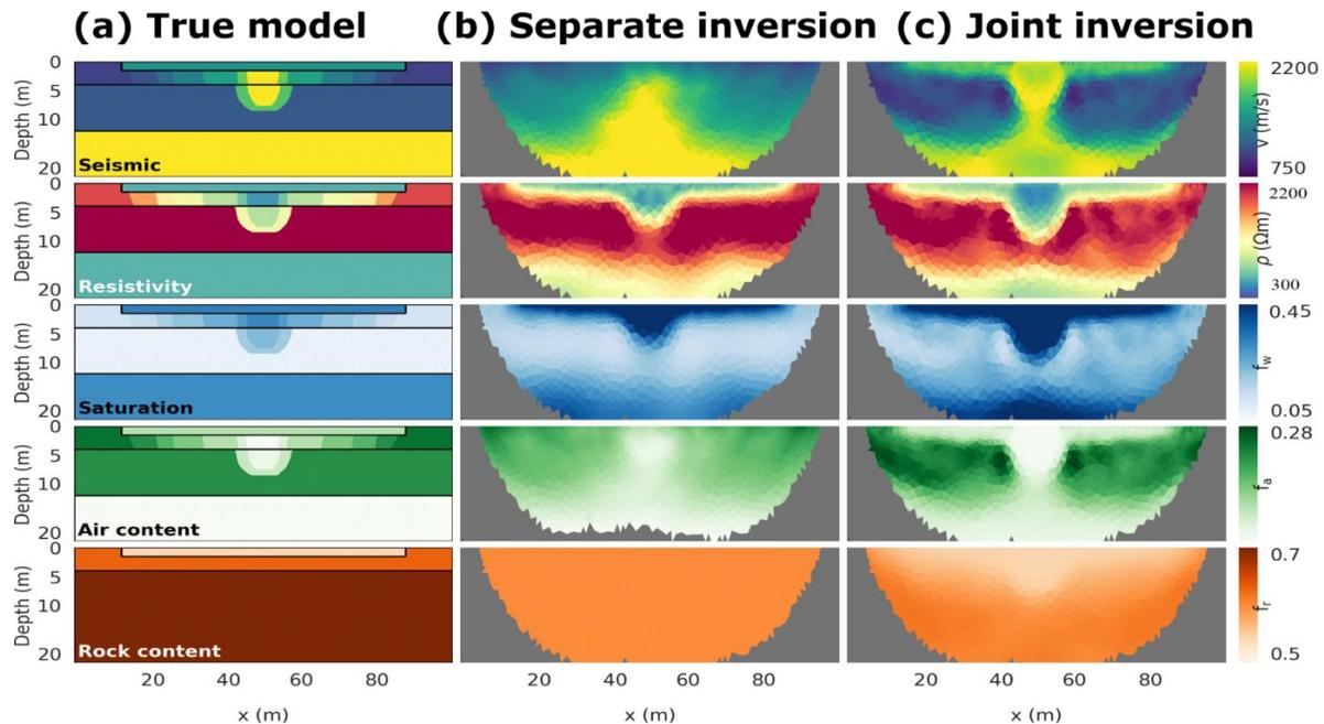
Figure 4 Numerical modelling for dry season river water recharge: seismic, resistivity, saturation, air content, and rock content models, from top to bottom.
