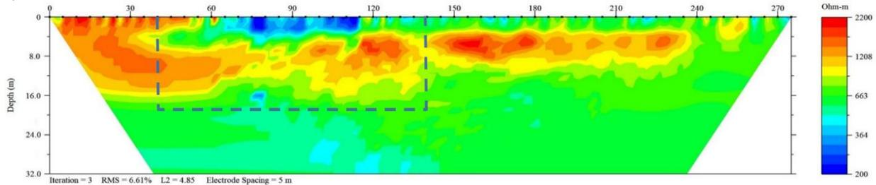
Figure 3 ERI inverted results for the dry season across the Choushui River. Numerical modelling for ERI and SRT joint inversion is performed for the dashed box zone.
