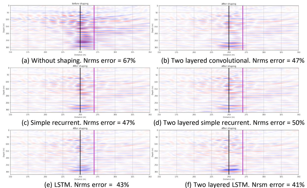
Figure 4. Reverse time migration differences between monitor and baseline. The black line in the center is the position of the VSP well. The magenta line is the approximate position of the CO<sub>2</sub> injection well.
