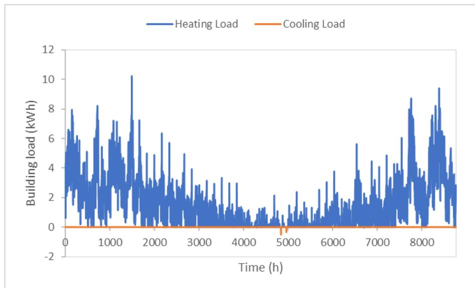
Figure 1 Hourly load profile of test site building, given insulation properties and a typical meteorological year in Alberta.
