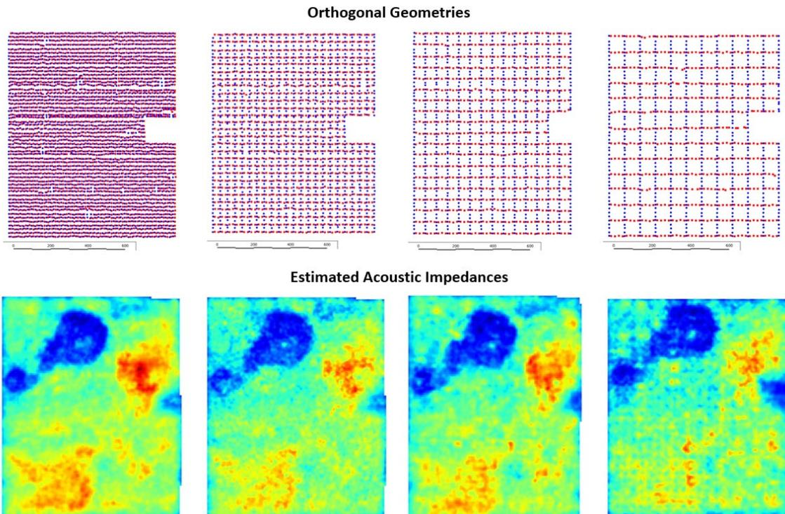
Figure 2: Comparison of Orthogonal Geometries with 20m, 40m, 60m, and 80m line intervals.
