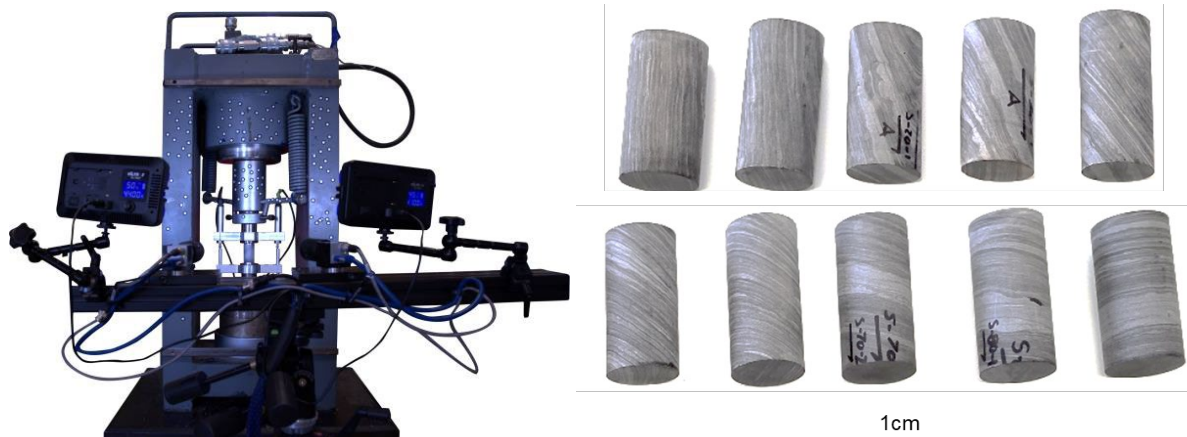
Figure 1: (a) UCS Testing Setup with Loading Frame, DIC, and LVDT (b) Example of Samples Cored at 0^{\circ} through 90^{\circ}
