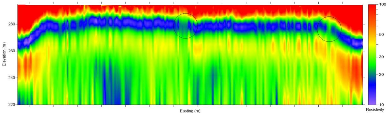
Figure 4. Cross section of TEM data moving east. Eastern and western edges of the section are shown sloping down.
