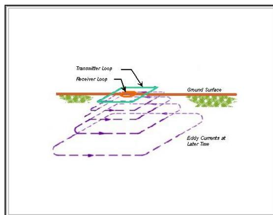
Figure 1. Centre loop TEM sounding configuration
