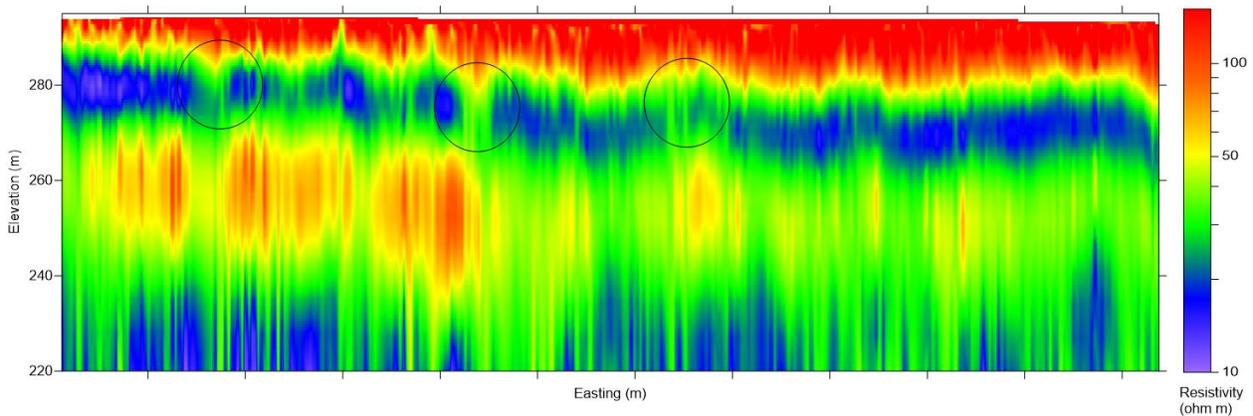
Figure 3. Cross section of TEM data moving east. Areas circled indicate zones of interest for possible hydrogeological pathways.
