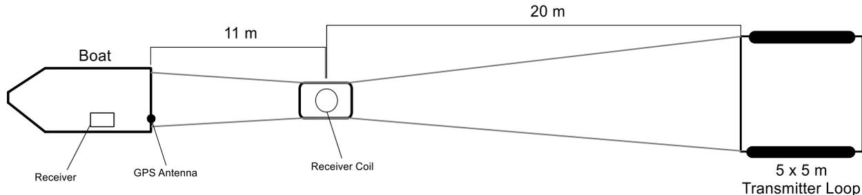
Figure 2. Marine TEM array schematic
