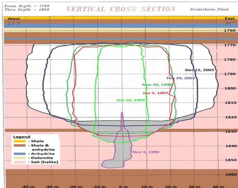
**Figure 1. Sidescan sonar plot of the existing salt cavern, 09-33-55-20W4. The colored lines indicated the progression of the cavern growth.**
