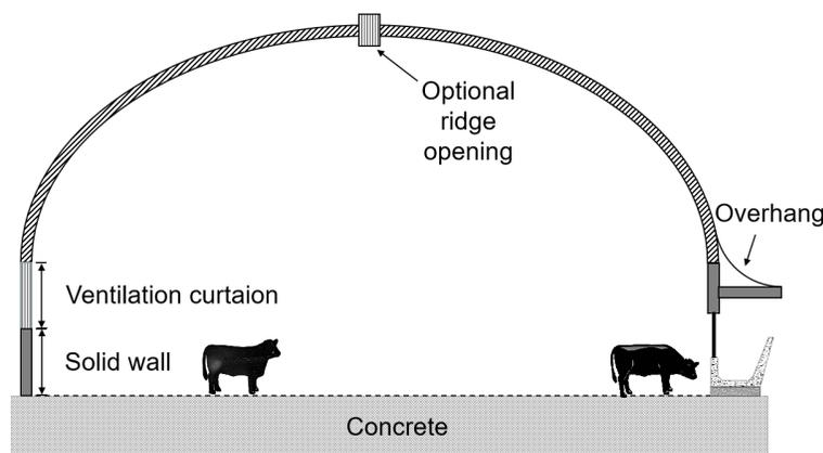
Fig. 1. Proposed feedlot pen design (modified from Honeyman et al., 2008).
