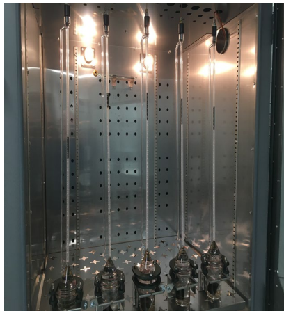
Figure 2. High-temperature Amott cell testing and oil recovery to determine superior surfactants.
