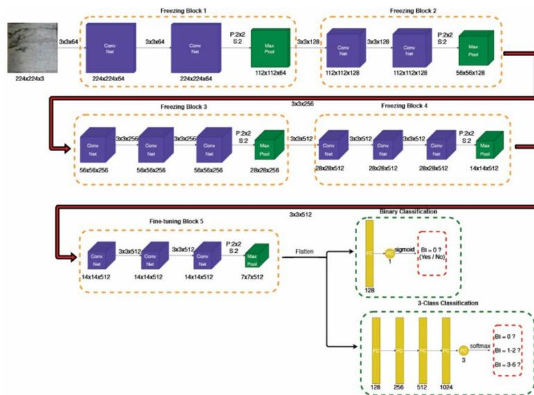
Figure 1. A convolutional neural network architecture based on VGG-16 with fully connected layers at the end. The architecture describes the routines for both binary and multi-class classifications. The input is a three-channel (red, green, blue) image. The binary classification problem outputs whether the input image is bioturbated or not. The multi-class classification problem outputs the class of the given image in terms of its bioturbation index range.
