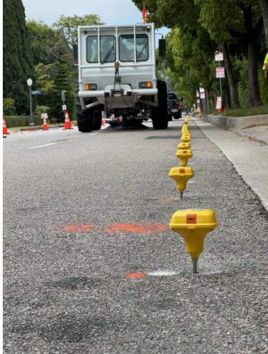
Figure 4 (Left): A typical seismic node. Note that everything is internal to the node weighing in at approximately 0.5kg.
