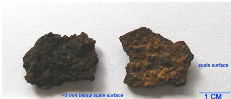
Figure 1: Goethite (Iron Oxide-Hydroxide) scale found in wellbore (Hudspeth, et al., 2023).
