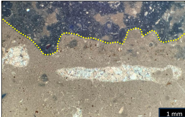
Figure 2. Photomicrograph displaying high porosity Thalassinoides isp. (delineated by the segmented, curved yellow line) contrasting the completely calcite-cemented Chondrites isp. below.
