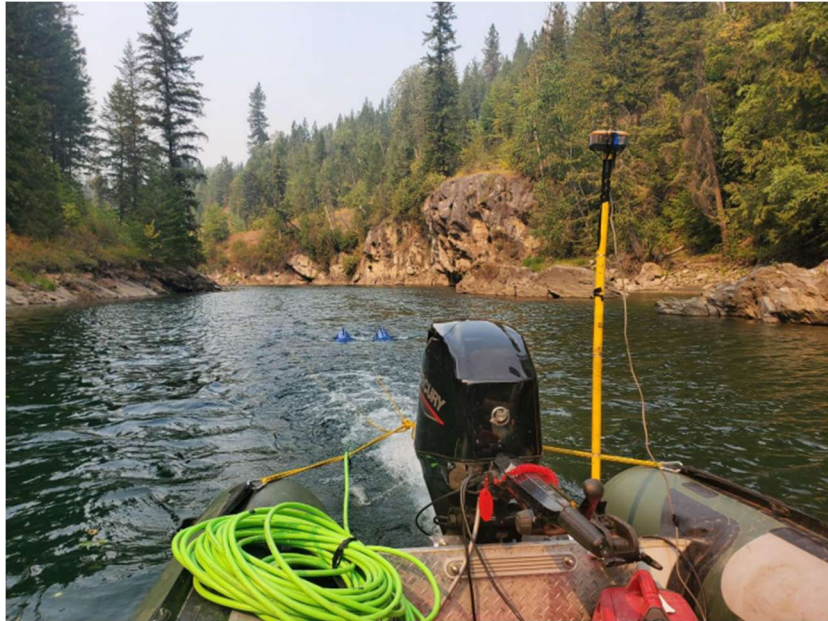
Figure 3: CHIRPceiver system being towed along the river, Geode GNS system (yellow) collecting GPS coordinates.
