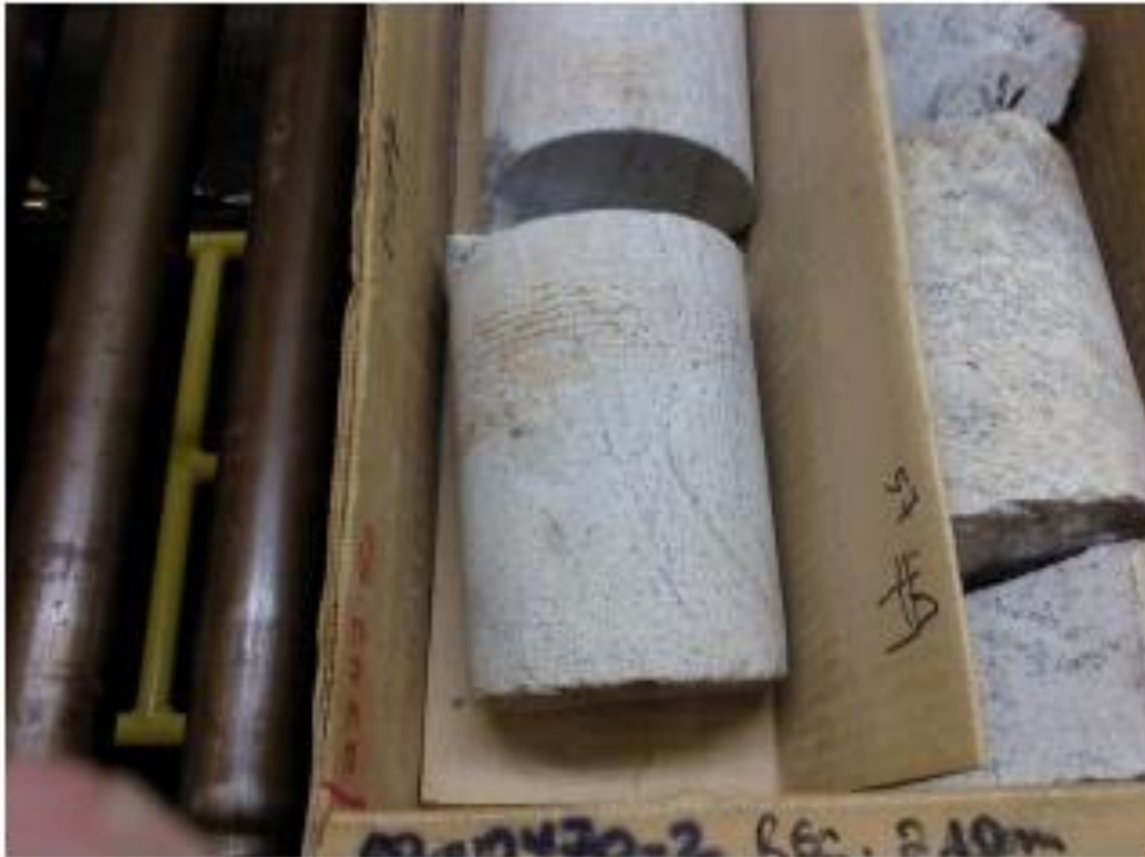
Figure 2. Granitic core from the deepest section of the Hunt Well (below 2,300 m, 7,590 ft). The diameter of the core is 4 inches (10 cm). Note the absence of fractures, this granite is totally tight. From: Majorowicz, J., et al, 2014, Geophysical Journal International .
