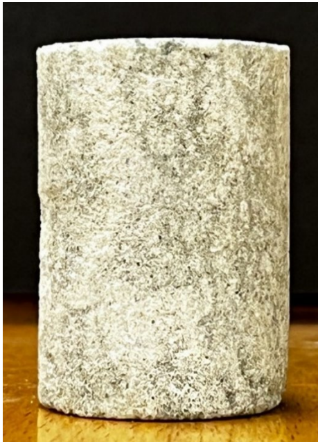
Plug 1, sandstone is intercalated with clay laminae and thin shale beds. This plug has porosity of 11.9% and permeability of 0.13 mD.
