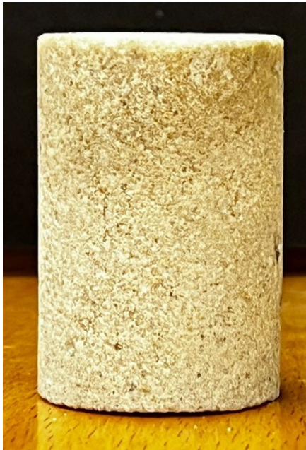
Plug 2, poorly sorted, semi-angular, coarse to granular quartz arenite. Scatter shiny spots may be iron-rich minerals such as pyrite. This plug has porosity of 14.1% and permeability of 102 mD.
