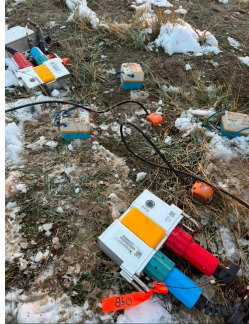
Figure 2. Example of receiver station with multiple collocated sensors with tailored gain settings.
