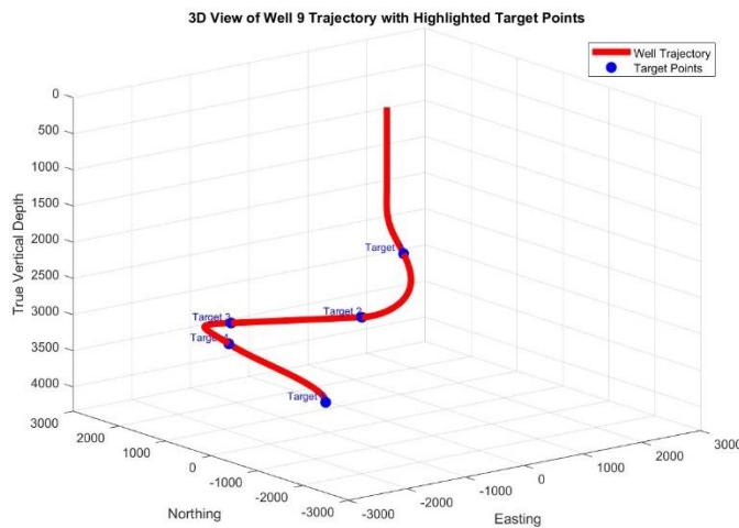
Figure 1: 3D View of generated well path
